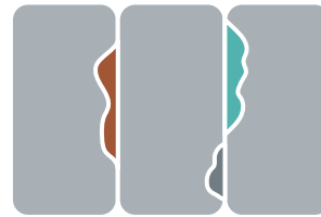
Galvanic corrosion occurs when different metals touch
