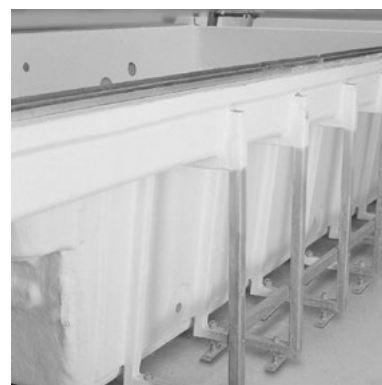
Wall bracing for channel basins self-supporting
