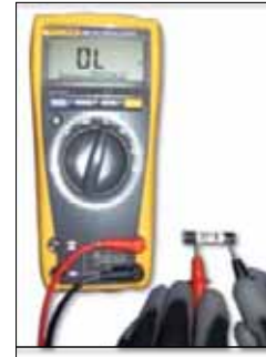
A FUSE WITH THE METER READING "BAD"
