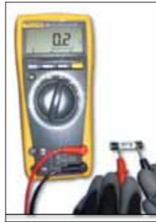
A FUSE WITH THE METER READING "GOOD"
