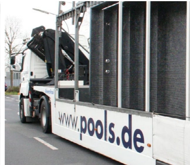
The pool is prefabricated in our factory, not on site. It is delivered to your location with a special transporter, either upright or on its base. Pools in segments are also possible - the flange is reworked on site with mosaic.
