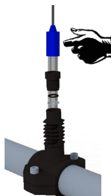
Step 22 Slide the nut onto the probe and the clamp underneath, then place the probe.
