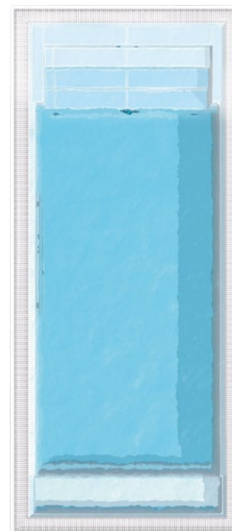
Overflow channel with stone cover adjustable overflow weir of V4A
