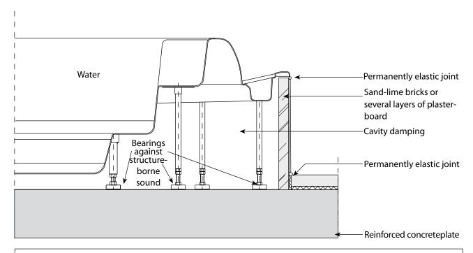
This recommended installation will only suffice as long as there are no rooms requiring protection to VDI4100/DIN4109 located below or adjacent to the installation room.
